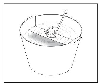
Figure 43. Testing the Oil Temperature Switch
